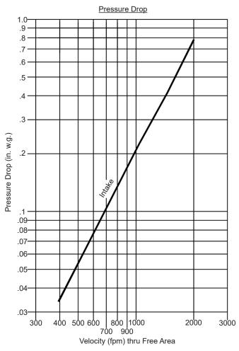
Intake air converted to standard air density.
